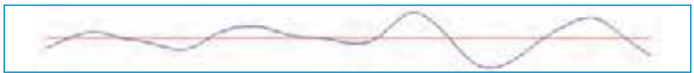
Fig. 4: Waviness profile after \lambda_c low-pass filtering and \lambda_f high-pass filtering with center line representation according to EN ISO 4287
